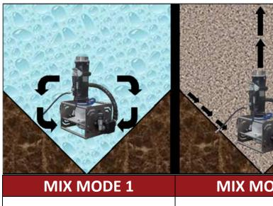
Use mix mode when there is fluid in the tank and the solids are on bottom.
